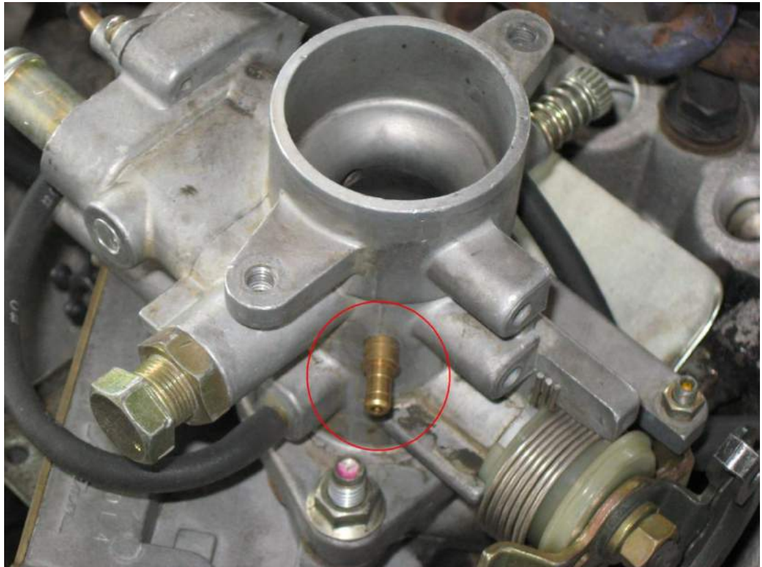
Figure 4b: Aisan Mixer – Location of vacuum port
